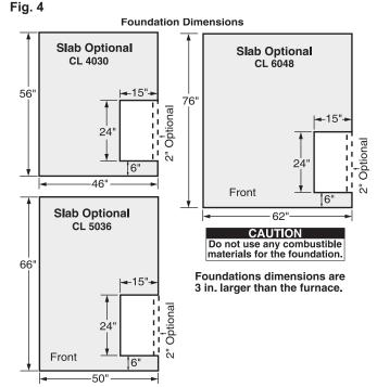
Outdoor furnace must be installed on a noncombustible surface or foundation that incorporates an enclosure that will prevent supply and return lines from possible exposure to sunlight, fire, or physical damage that may be caused by an occurrence outside the outdoor furnace enclosure. Foundation may consist of concrete, crushed rock, or patio blocks.
