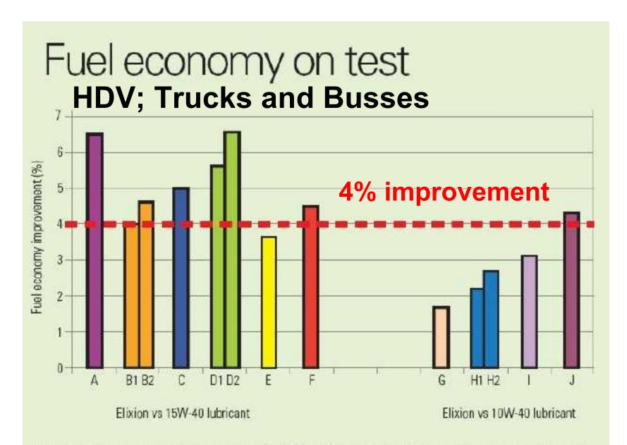
The graph shows the result of an extensive series of field trials carried out on fleets of commercial trucks and buses (plotted as A-J above). Elixion, BP's heavy duty diesel engine lubricant, was used in the trials, and consistently demonstrated improved fuel economy compared with conventional engine lubricants, giving an average improvement of around 4 per cent (red dotted line)
