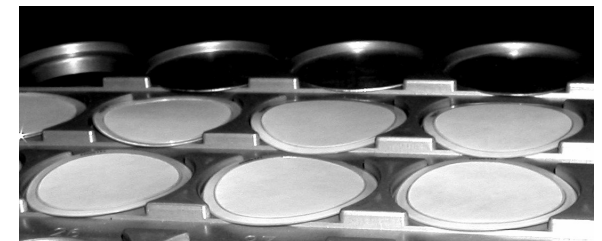
Fig. 2 Filters set up in the weighing tray ready for weighing.
