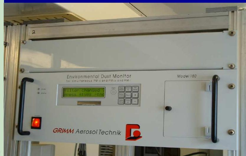
**Simultaneous measurement of PM<sub>1.0</sub>, PM<sub>2.5</sub> and PM<sub>10</sub>**
