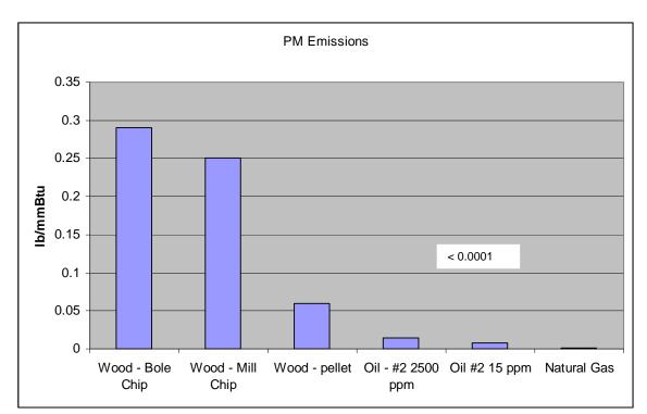
Figure 2. Fine particle emissions rates for wood- and oil-fired commercial boilers.
