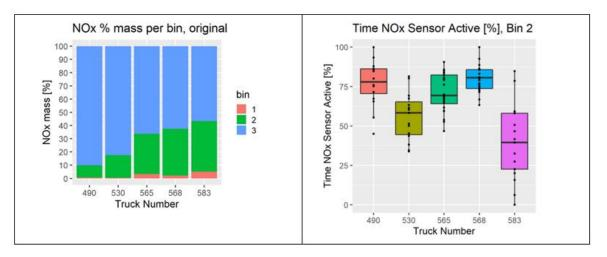
*Figure 6:* NOx mass in bins 1, 2, and 3 (left); and time NOx sensors were active in bin 2 for each of five trucks data logged (right).
