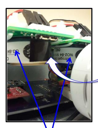
Alphasense B4 Electrochemical O<sub>3</sub>, CO, NO & NO<sub>2</sub> Sensors (\$216 ea.)
