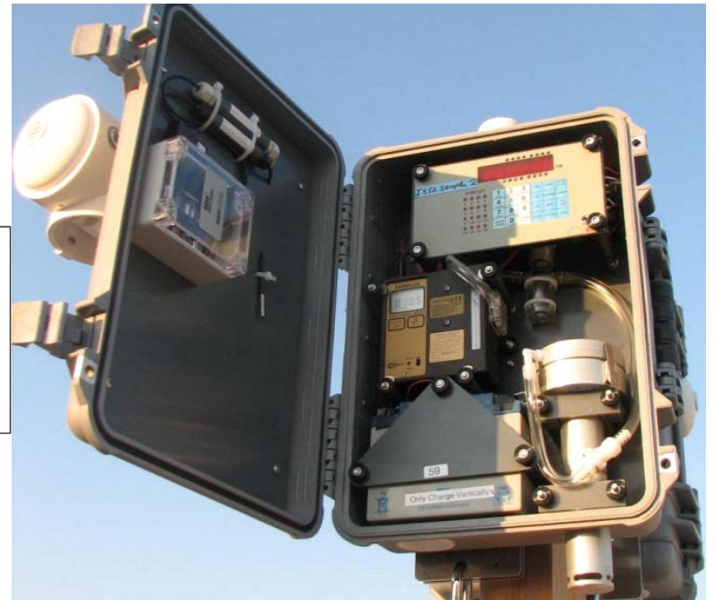
NO x , NO 2 , SO 2 , and O 3 are collected with passive monitors in a protective housing
