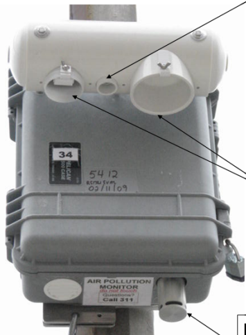
Temperature/RH sensor data logger records temperature and relative humidity.
