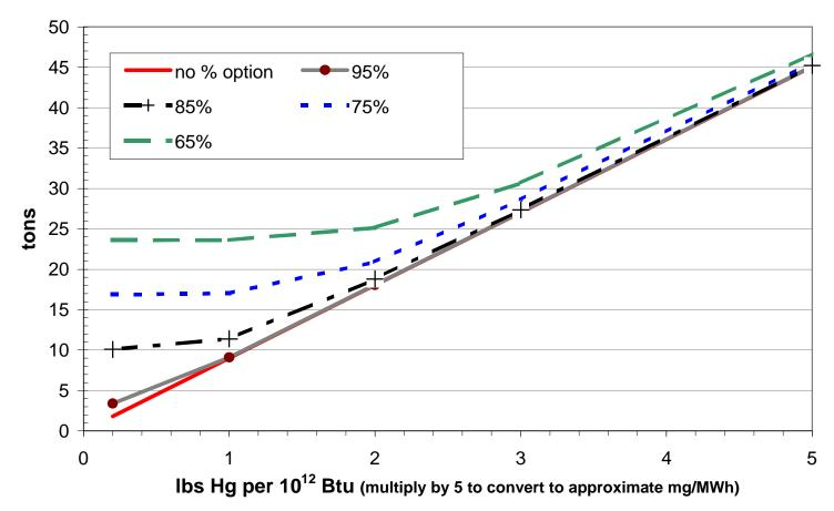
Note: Plant by plant emissions were estimated for various combination standards in the form of <u>A</u> lbs. per trillion Btu or <u>B</u> percentage reduction of mercury (based on coal mercury content), whichever is less stringent, with the assumption that a plant's emissions will reflect the less stringent applicable standard. Estimated emissions for all plants were totaled. Data source is the same as Appendix 1.
