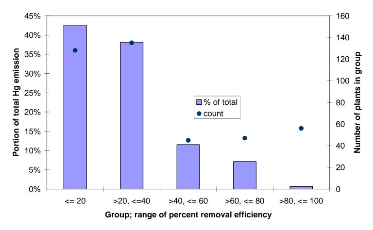
Note: Data source is the same as Appendix 1. Percent removal efficiency was based on comparison of USEPA estimated plant by plant emissions compared with total mercury content of coal purchased by that plant, as estimated from the quarterly coal data files.
