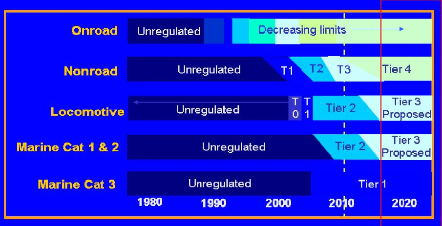
Tier 0 locomotive standards apply retroactively to engines built since 1973, upon remanufacture.
