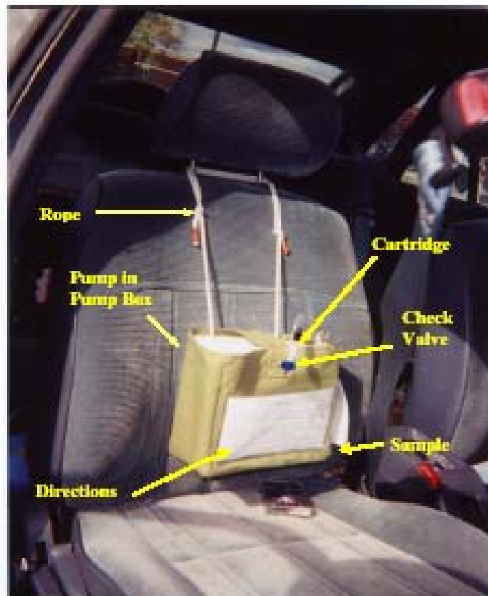
Figure 2. In-vehicle sampling setup as it was placed during sampling.
