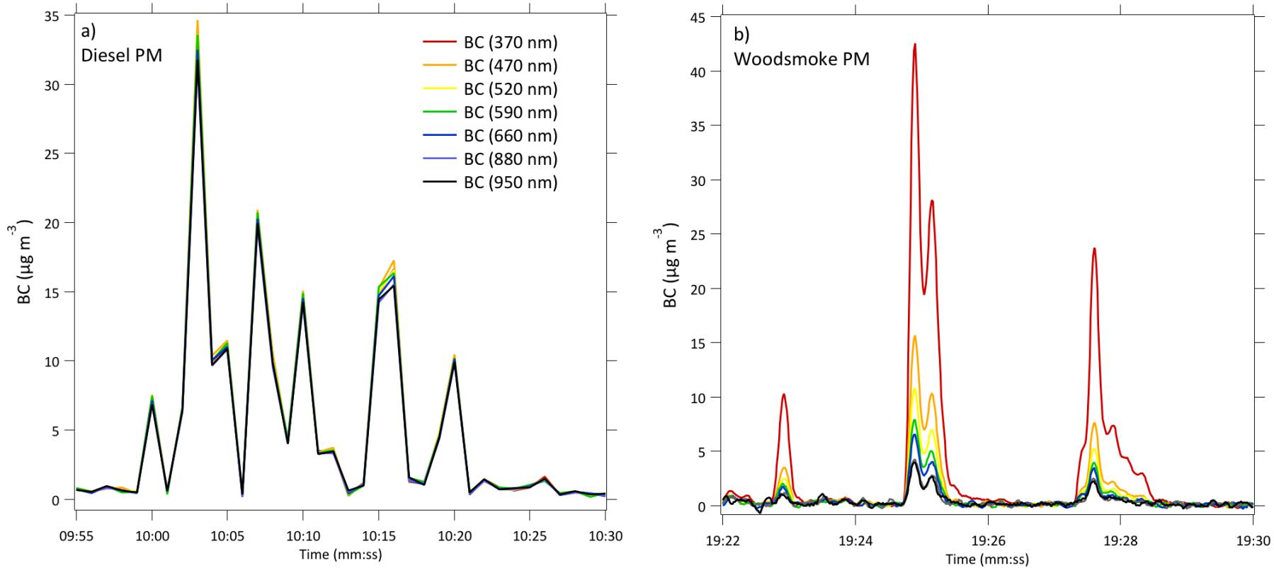
Diesel PM: No enhancement for UV absorption
