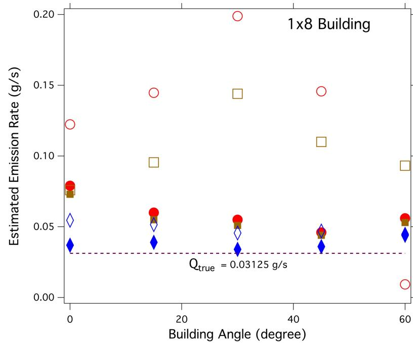
Model 1: Gaussian Plume (GP) Equation Use the Dynamically Dimensioned Search (DDS) algorithm to fit the equation with measurements to determine the parameters Q (emission rate),  $\sigma_y$  and  $\sigma_z$  (vertical and lateral dispersion coefficients),  $h_{eff}$  (effective height) and  $\delta y$  (lateral offset).
