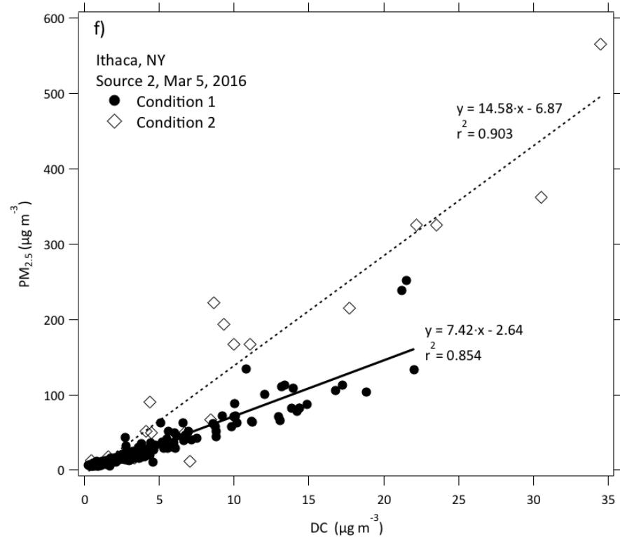
Different PM vs. DC relationships indicate different combustion conditions
